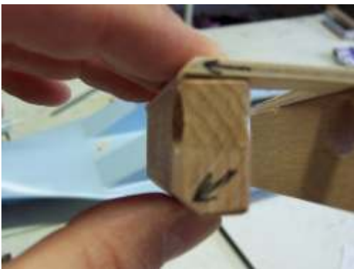
Rounded off edges to match fuselage contour
