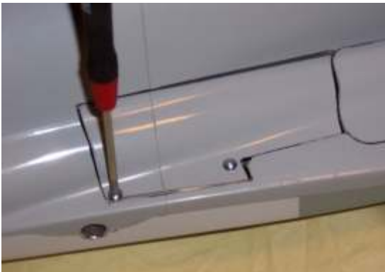
Cut out glass fibre used as wheel door
