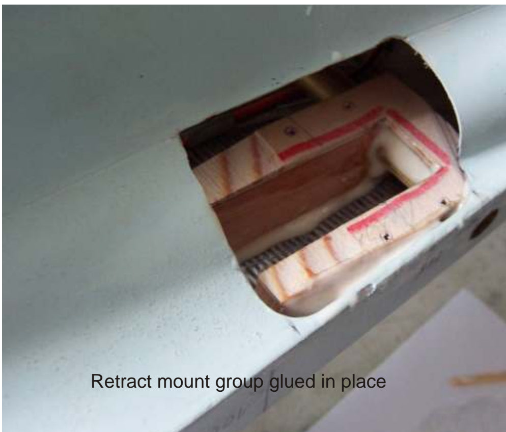
Rounded off edges to match fuselage contour
