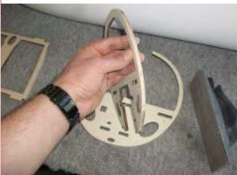
Sand off the burned surfaces on the formers
